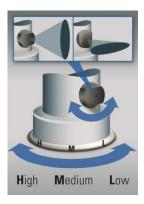
The spray head is doubly rotatable. By turning the small black nozzle the spray cone can be precisely controlled. By turning the whole spray head to the positions Low, Medium, High, the spray quantity can be regulated.
