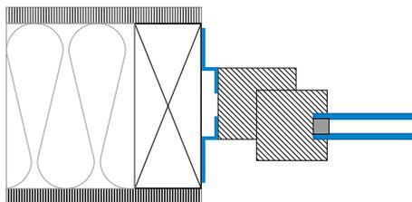
**Principle:** Both adhesive tapes before window installation. Alternating bonding.
