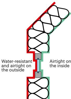
A building connection will retain its function in the long term if the layer on the inside and the windtight and driving rain impermeable layer on the outside are joined permanently and without gaps. This requires the creation of a sealing system with sufficient freedom of movement. This principle is used for window connections.
