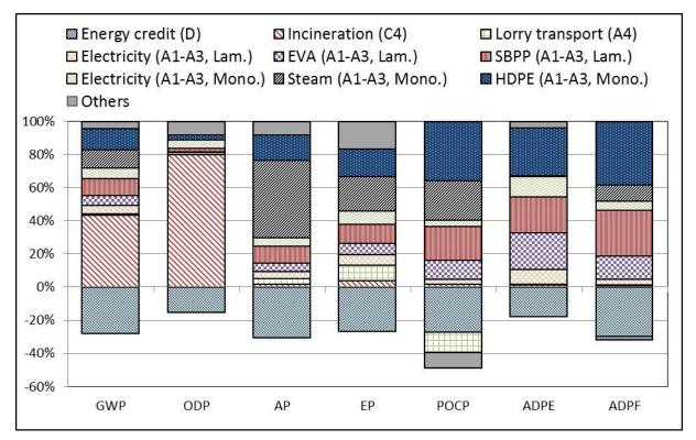
For most of the impact categories, more than 70% of the impact is dominated by the functional layer (HDPE granulates and steam supply mainly) and lamination (SBPP supply mainly) production steps; except for **ODP** which is dominated by the incineration of the product after its use.
